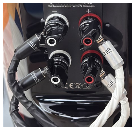
The WBT bi-wiring terminal has new wing screws and allows for high clamping pressure.
